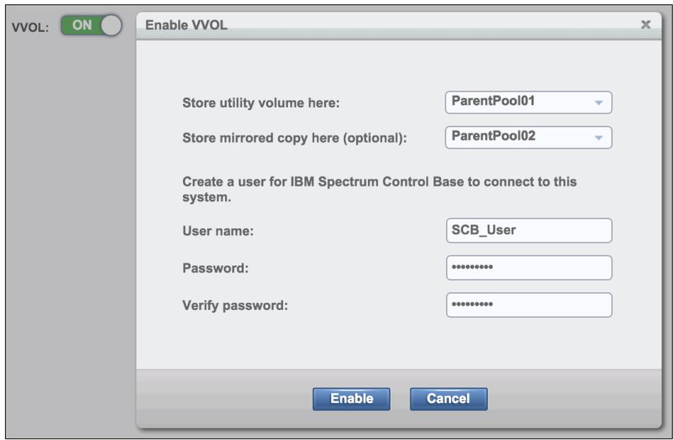
Figure 3 Storage system: Enable VVOL dialog
