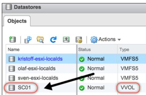
Figure 33 vSphere Web Client: VVol datastore
